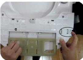
4. Put the fixing plate, adjustment pads and adjustment sheet metal plates orderly on the toilet.
